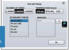
RTD can be connected with 2, 3 or 4 wires and you can select various tables such as the IEC 60751, JIS or Callender Van Dussen
