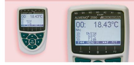
ALMEMO<sup>®</sup> professional measuring instrument with data logger function.
